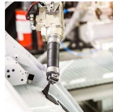
Weight-saving, clean and efficient: automated application of LASD.
